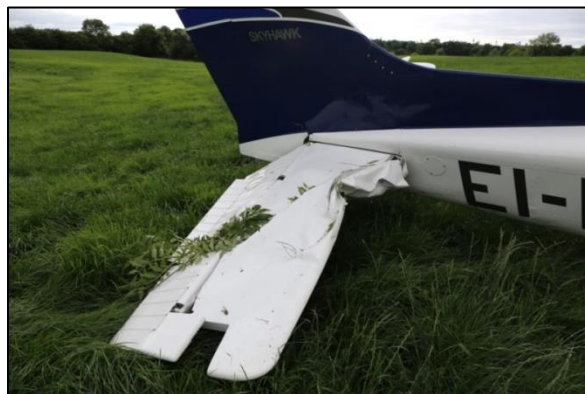
Photo No. 3: Impact damage to right horizontal stabiliser
