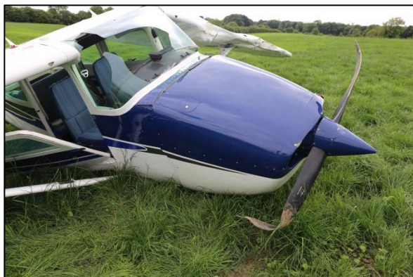
Photo No. 2: Damage to propeller blades; engine cowling and mounting points; windscreen; and right-hand access door
